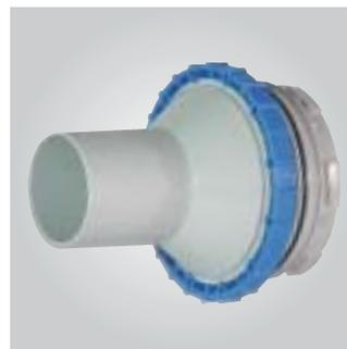
BKD 150 sealing collars will be supplied fitting to the wall thickness of the structural works and are inserted flush into the formwork. (L = wall thickness in mm)
