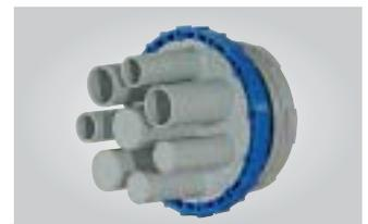
System cover with 8 connection pieces and 4 shrink-on sleeves. 4 connection pieces are closed upon supply and can be opened when necessary. Suitable for max. 4 cables of diameter 7 - 23 mm and max. 4 cables of diameter 12 - 33 mm.
