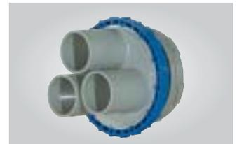
System cover with 3 connection pieces and 3 shrink-on sleeves. Suitable for 3 cables of diameter 21 - 56 mm. Several joint boxes AK or sealing plugs VS 60 (as blind cover) are available as accessory.
